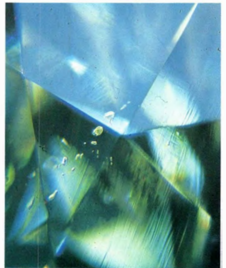
Internal graining (caused by strain in the crystal) and crystals in a diamond from Argyle, Western Australia. Photo: B. Sechos.
