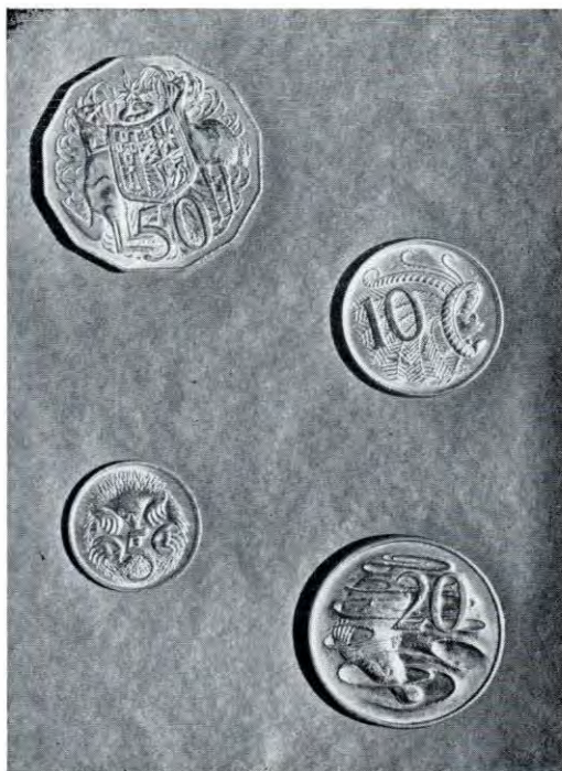
Australia's 5, 10, 20, and 50 cent coins are cupro-nickel (75 per cent copper, 25 per cent nickel). [Photo: New South Wales Department of Mines.]
