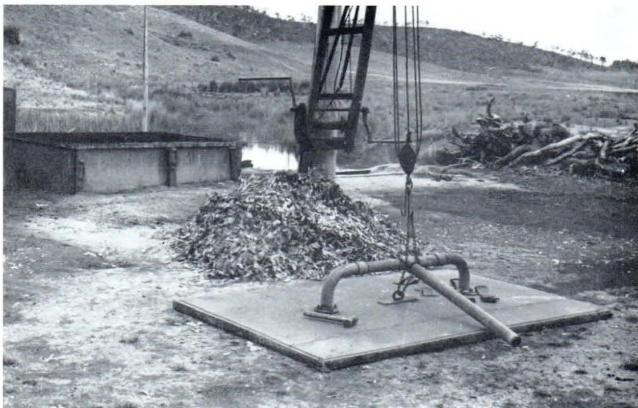
A distillation plant used for the production of Eucalyptus dives oil in the Braidwood district, New South Wales. A heap of leaves may be seen, ready for charging into the still. When the still is full the heavy lid in the foreground will be lifted into position by the crane. The stream behind the still cools the condenser. At right is a heap of firewood to fire the still. [Photo: J. L. Willis.]
