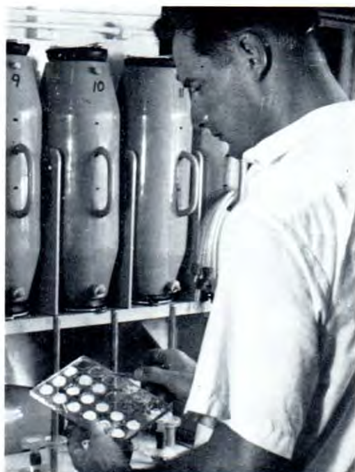
A C.S.I.R.O. scientist at work in the laboratory of one of the Australian oceanographic frigates. The bottles in the rack contain samples of sea-water from various depths. These samples are filtered through fine "millipore" membranes (in the tray) and the concentration of activity of minute phytoplankton organisms measured. [Photo: Commonwealth Film Unit.]
