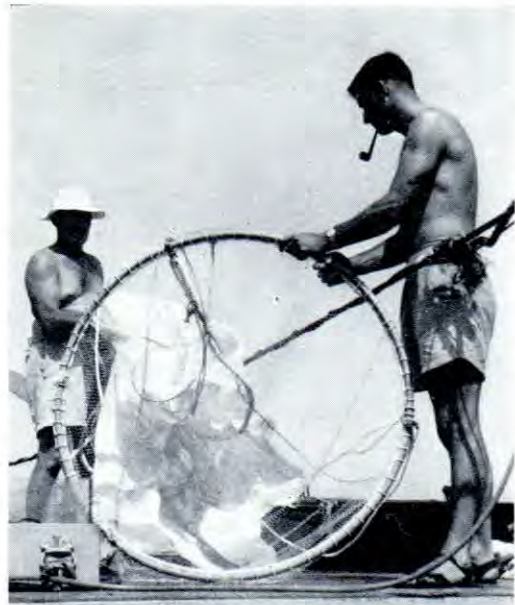
The Indian Ocean Standard net, adopted for general use in the expedition. This is a nylon net with a mouth area of one square metre. It is hauled vertically from 200 metres to the surface. [Photo: Commonwealth Film Unit.]
