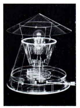
A transparent plastic light-trap designed to collect mainly soft-bodied insects, such as moths. The diameter at the base is 18 inches. The hood is only used during rain to protect the mercury vapour lamp. [Photo: C. Lourandos, C.S.I.R.O.]
