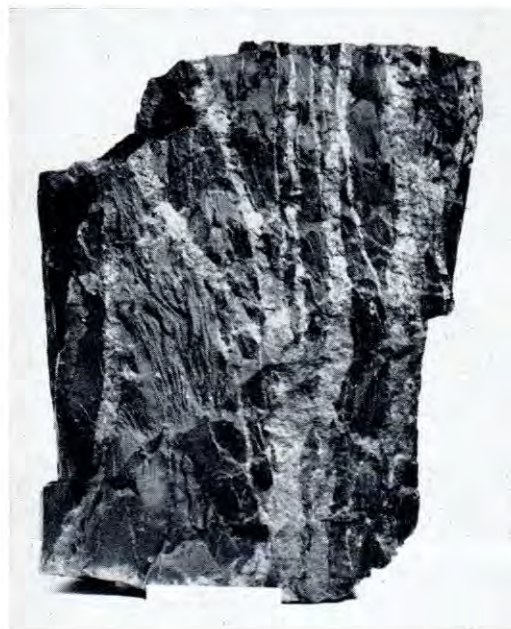
Typical primary copper ore from the Great Cobar Mine, showing veins of chalcopyrite-pyrrhotite-magnetite and quartz in slate.
