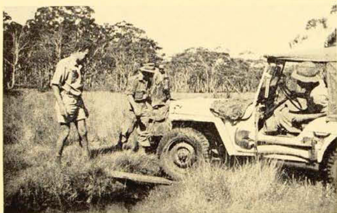
Negotiating swampy areas on the Snowy Plains. Deep but narrow swamp gutters are bridged with planks.
