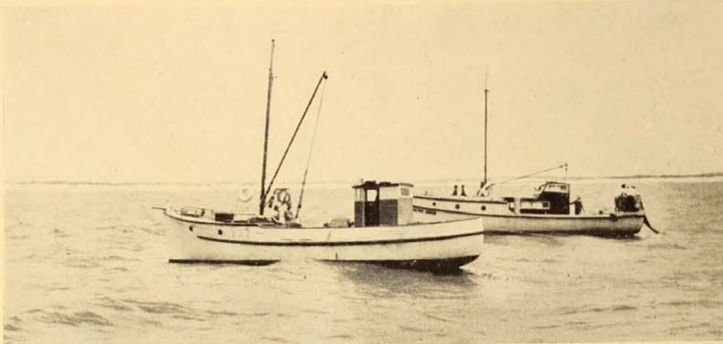
Converted seine-net fishing trawlers operating off coast at Evans Head, New South Wales. Crew of craft at right are pulling inboard the cod end of an otter trawl filled with prawns.
