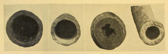
End view of four water pipes. On the left is a new type of iron piping lined with bituminous compound to prevent the workings of iron bacteria. Alongside it is an unused iron pipe for comparison with the next one, which is regular iron pipe badly affected by iron bacteria. On the extreme right is an old style lead pipe; it is unaffected by iron bacteria even after seventy years of service.
