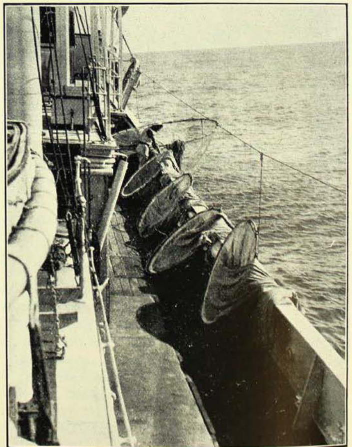
The five nets ready to be lowered overboard and towed at intervals of 1,000 metres of wire to secure specimens of deep-sea creatures. The large three-metre net is the first to be put down.
