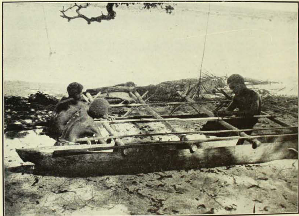
Repairing a small fishing canoe of the outrigger type (wang). [Photo.—F. L. S. Bell.]
